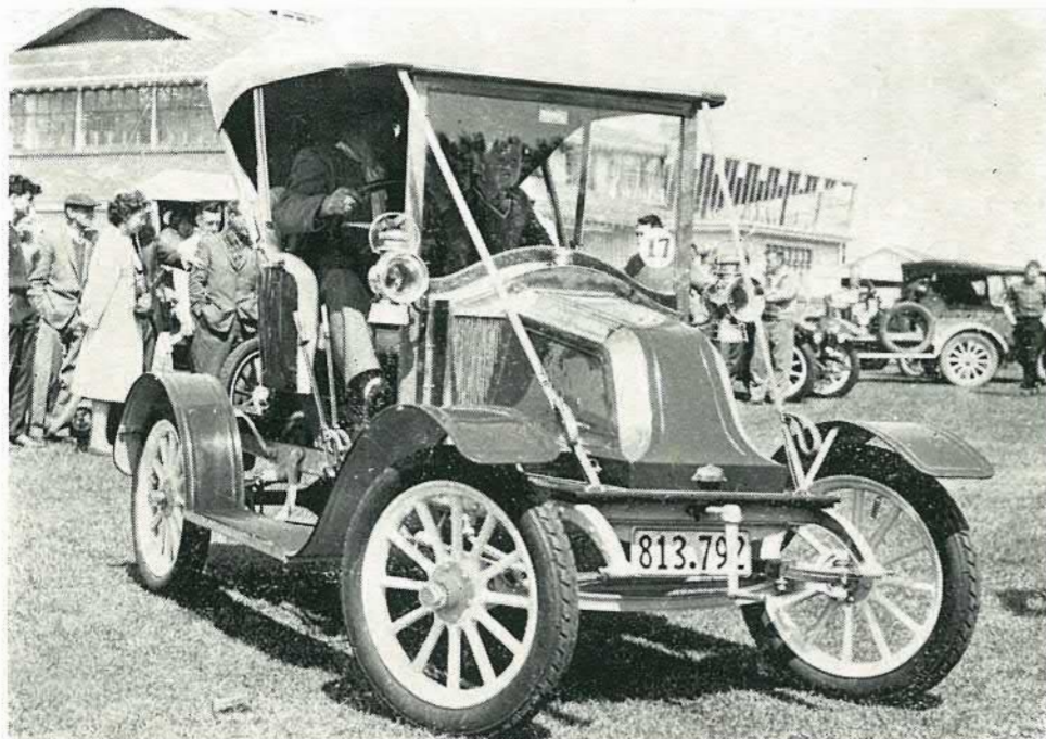
Derelict when Mr J. Cooper took it over, this two-seater 1910 Renault now represents five years of restoration work. The car, an 8 h.p. two-cylinder model, is but one of many excellent vintage cars owned in Christchurch.
